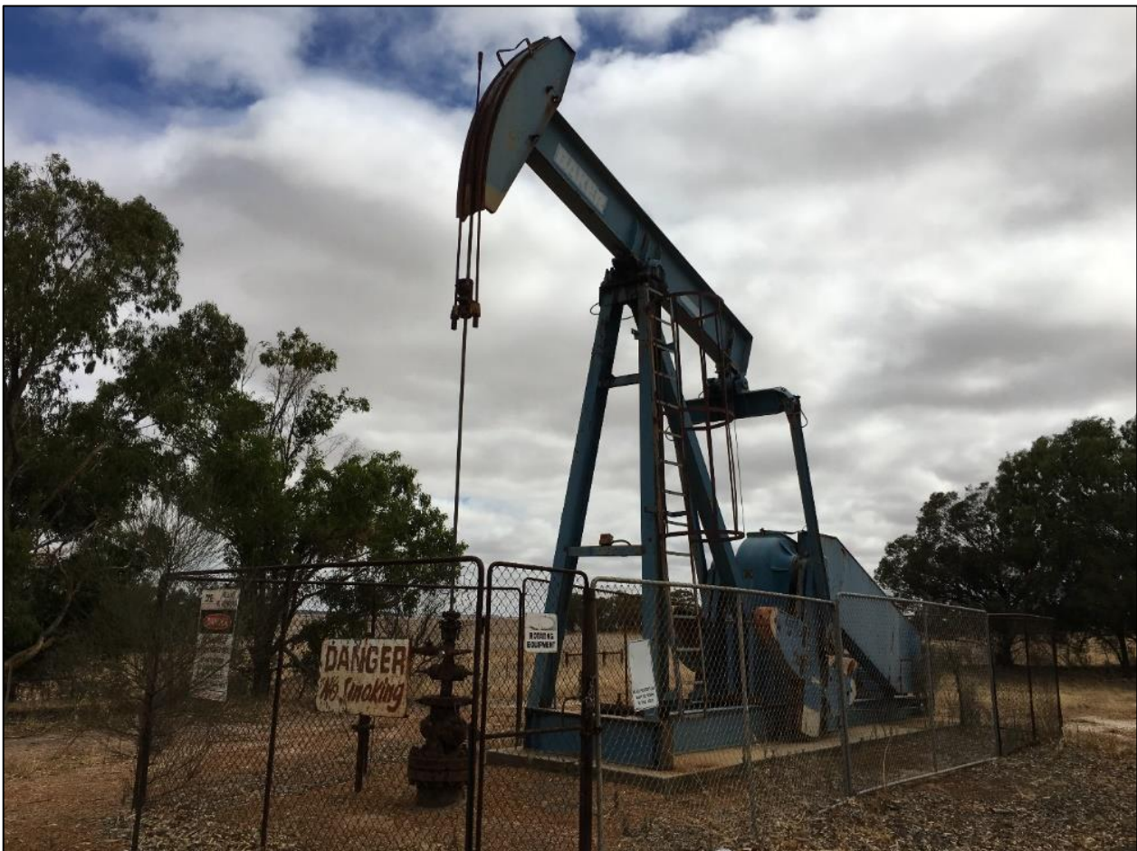
Potential workover candidate - Mount Horner-5A Well head and beam pump
